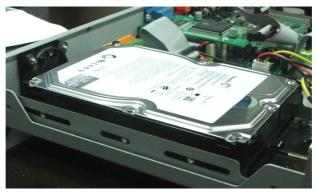
D. Fix the harddisk on the support with screw, and cover the DVR.
