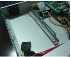
B. Connect the harddisk data and power cable well
