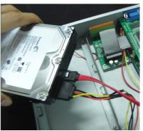
C. Put the harddisk into support, and align the harddisk's screw hole with the support.
